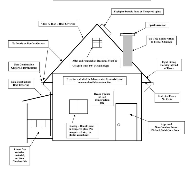
No vinyl or plastic handrails on decks unless approved & fire rated
